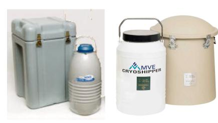
Different models of dry shippers. Shown in each picture is a transfer case with the inner Dewar taken out.
