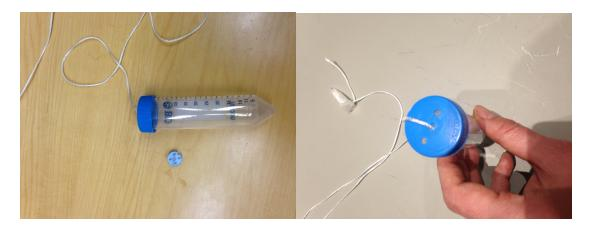
Falcon tube with a string for retrieval. Holes are made on the lid and/or on side of the falcon tube so that  $LN_2$  can go in when immersed in liquid nitrogen.
